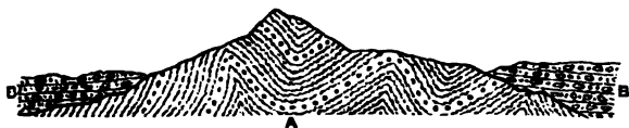
FIG. 44.—Section of a mountain formed of crumpled rocks, A, which have been contorted before the deposition of the flat rocks, B.
